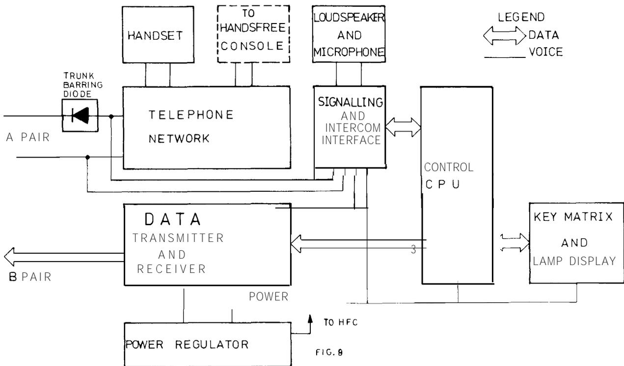
FIG. 8 - N308 TELEPHONE STATION BLOCK DIAGRAM
