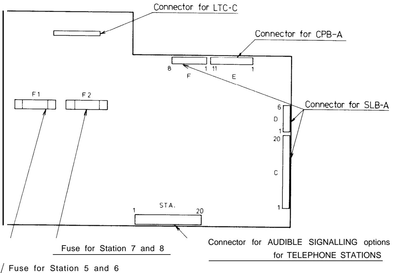
FIG. 42 - 4SB-A CONNECTOR LAYOUT
