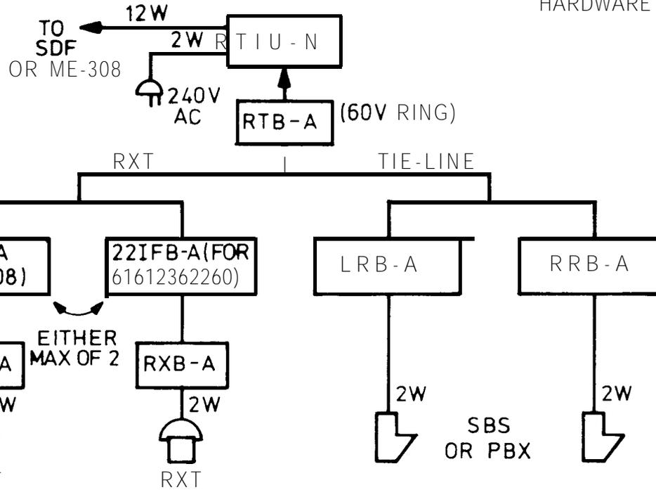
EACH RTIU-N CAN FEED TWO TERMINAL CONNECTIONS
