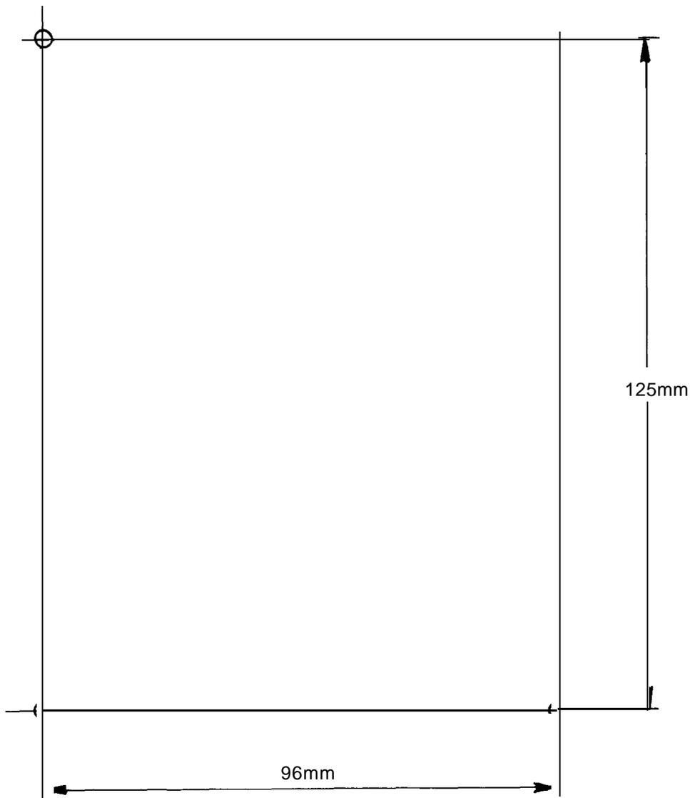
FIG 29A - WALL MOUNTING FOR THE TRUNK BARRING UNIT
