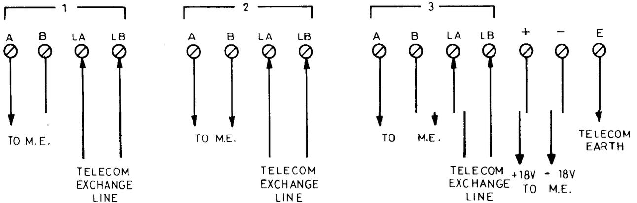
FIG. 36 - CALL METERING UNIT WIRING
