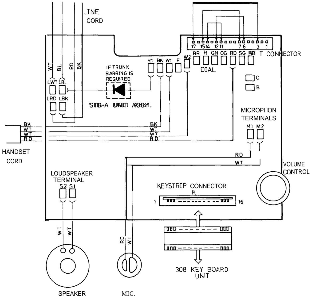
FIG. 34 - STB-A STATION BOARD ASSEMBLY
