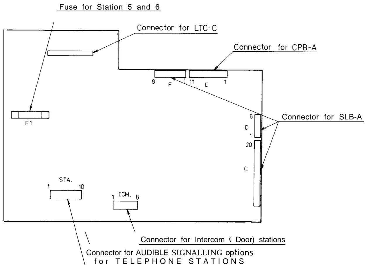
FIG. 43 - SIB-A CONNECTOR LAYOUT
