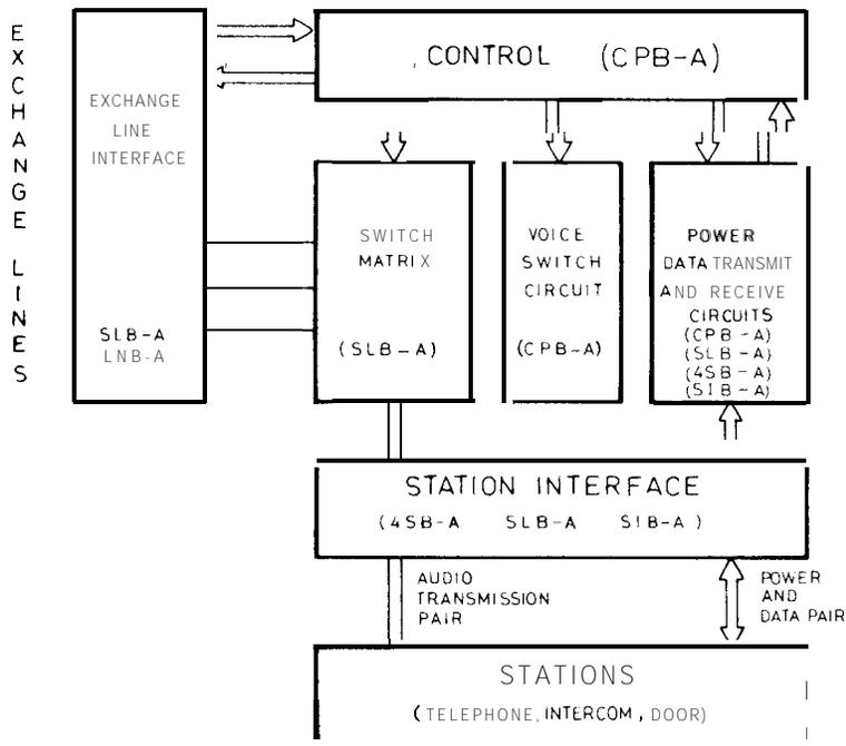
FIG. 7 - N308 MAIN EQUIPMENT BLOCK DIAGRAM
