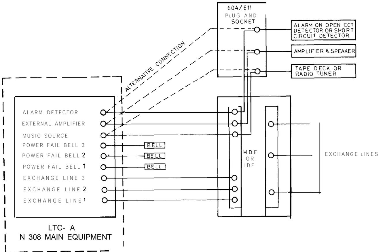
FIG. 30 - TERMINATING OF SYSTEM
