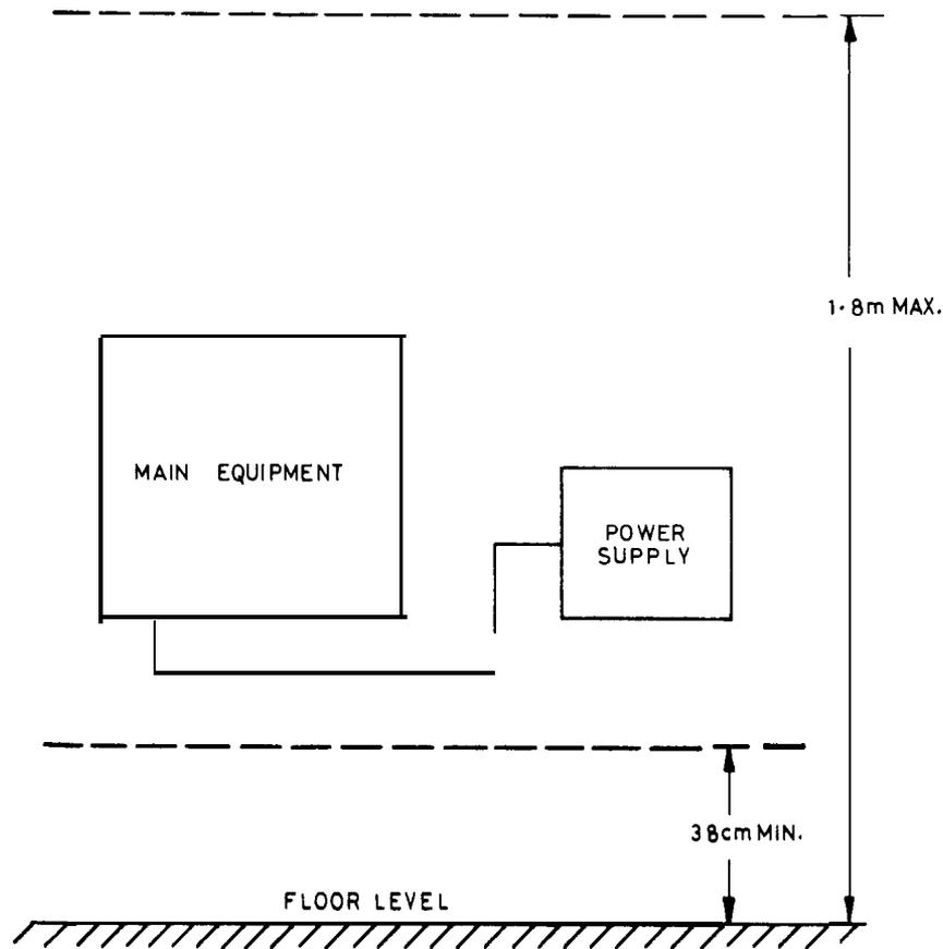
FIG. 25 - LIMITATIONS ON WALL MOUNTING
