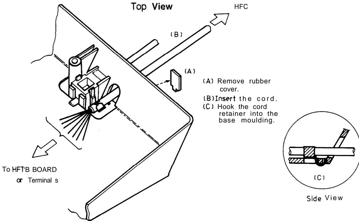
FIG. 37 - HANDSFREE CONSOLE CABLE INSTALLATION
