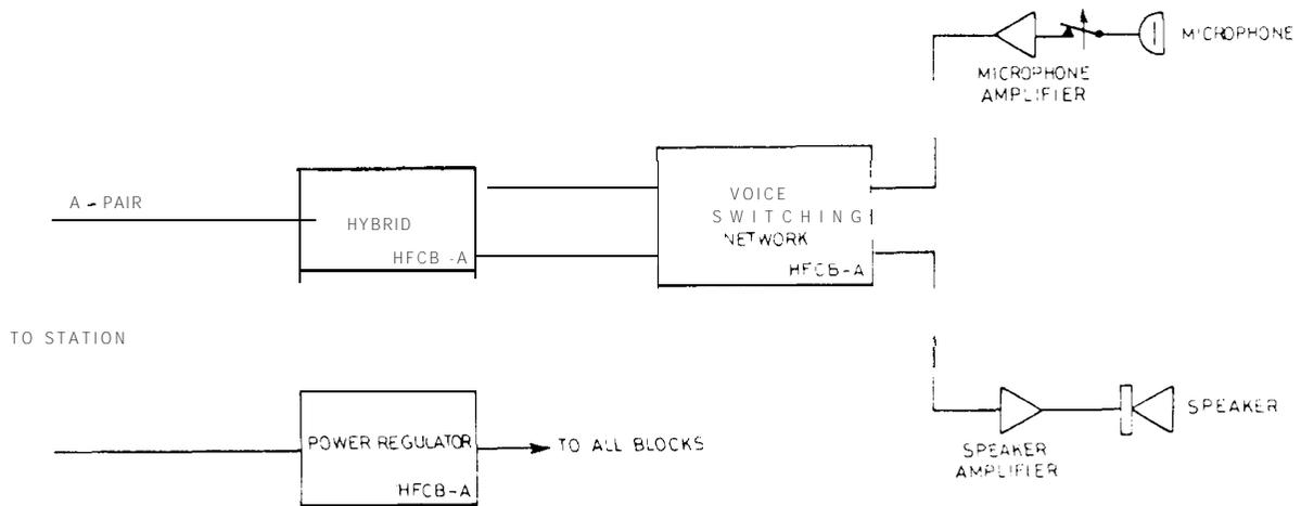
FIG. 10 - HANDSFREE CONSOLE BLOCK DIAGRAM
