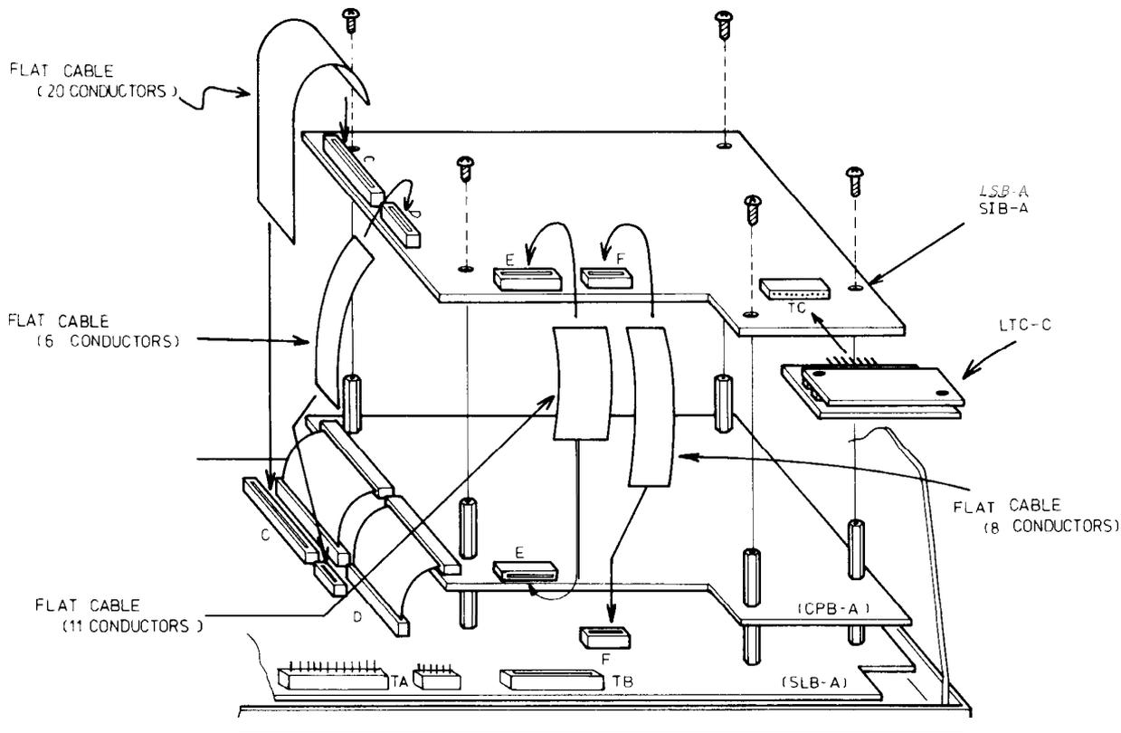
FIG. 31 - EXPANSION BOARD INSTALLATION
