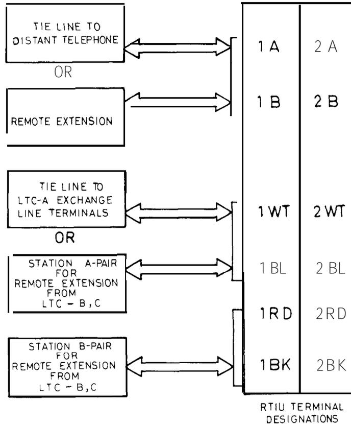
FIG. 33 -RTIU TERMINAL CONNECTIONS
