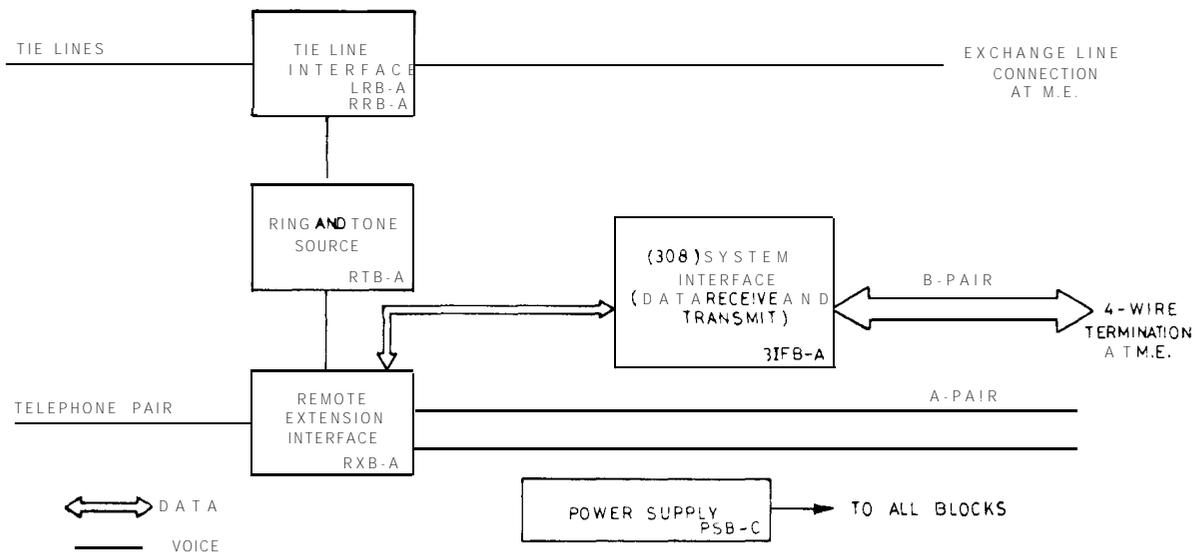
FIG. 11 - REMOTE EXTENSION AND TIE LINE INTERFACE UNIT BLOCK DIAGRAM
