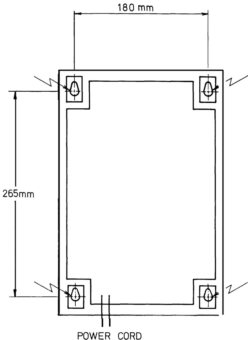
FIG. 26 - WALL MOUNTING OF MAIN EQUIPMENT
